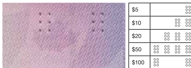
Figure 1: Raised-dot tactile feature
